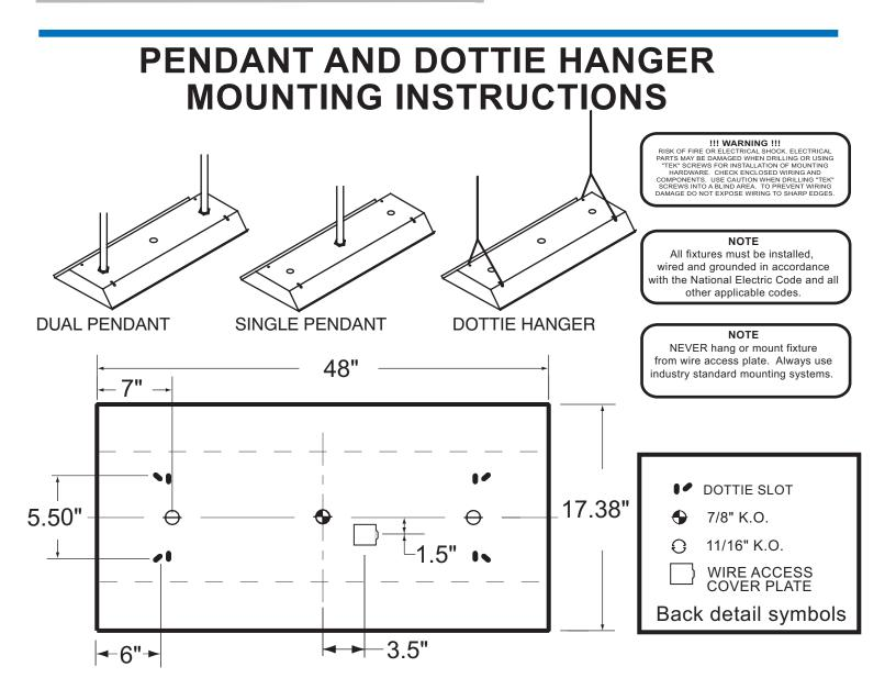
DUAL PENDANT MOUNTING - Remove two end 11/16" K.O.'s install pendants and secure using fasteners provided with pendant.
