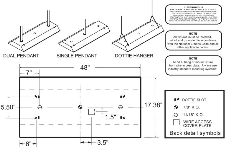
DUAL PENDANT MOUNTING - Remove two end 11/16" K.O.'s install pendants and secure using fasteners provided with pendant.
